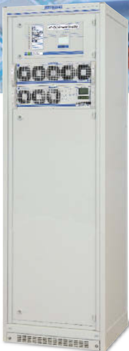
Fig. 8: Inverter- rectifier cabinet with: 3 inverter modules, static and manual bypass Total AC output power 4.5 kVA 5 rectifier modules output voltage 220V DC, output current 50A DC
