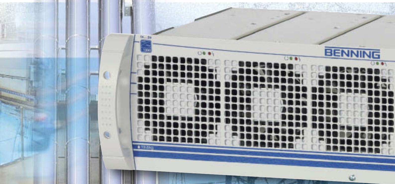
Fig. 5: 19" Sub-rack with 3 inverters, static bypass and manual bypass, output voltage 230 V AC, output power 4.5 kVA
