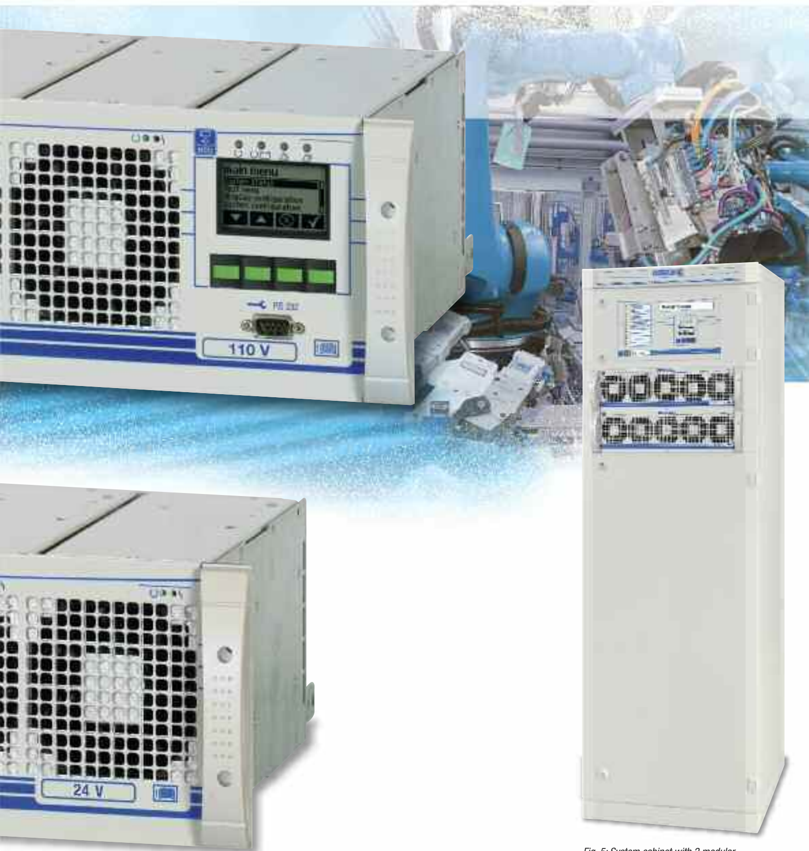
Fig. 5: System cabinet with 2 modular DC/DC converter plug-in units, output voltage 220 V, output current 100 A
